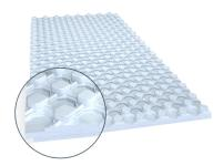
The **SR.HydroPex**<sup>™</sup> panels manufactured by Styro Rail<sup>™</sup> are composed of type 2 [200 series] expanded polystyrene [EPS] rigid insulation or type 3 [300 to 600 series]. A honeycomb-layout creates a spacing with intervals of 762 mm [3"] for the placement of the pipes. The system is compatible with all pipes dimensions: 13 mm [1/2"], 16 mm [5/8"], 20 mm [3/4"] and 25 mm [1"].
